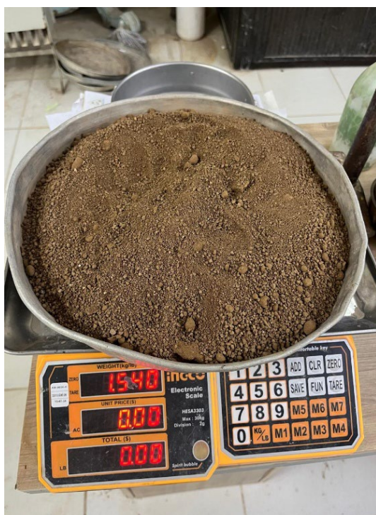
a) Weighing and preparation of oven-dried soil prior to contamination
