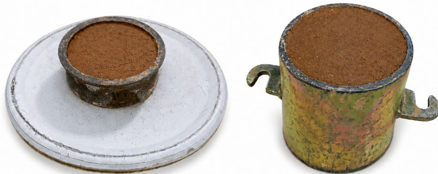
c) Remolded Samples of Consolidation and Permeability
