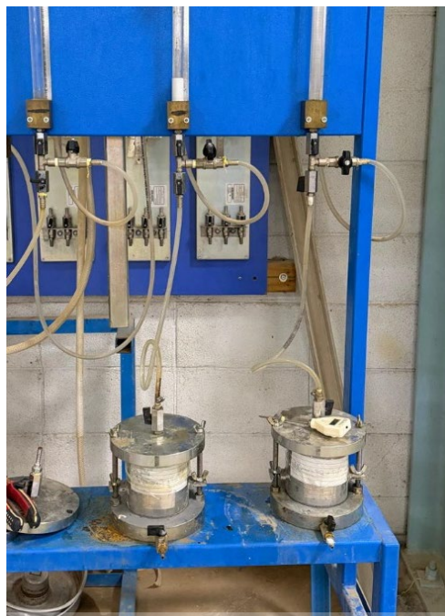
b) Falling-head permeability apparatus used for determination of hydraulic conductivity as per ASTM D5084.,
