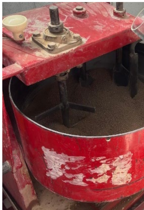
b) Mechanical mixing of soil and landfill leachate to obtain a homogeneous contaminated sample.
