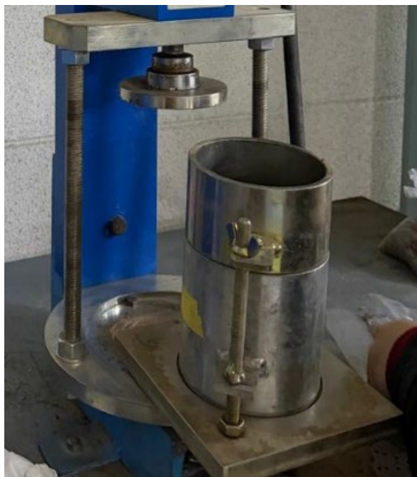
a) preparation and compaction of the remolded soil specimen in the permeameter mold
