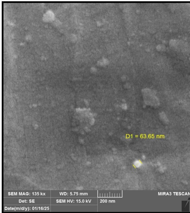
Figure 2: Water-acrylic based polymer curing compound SEM for surface morphology
