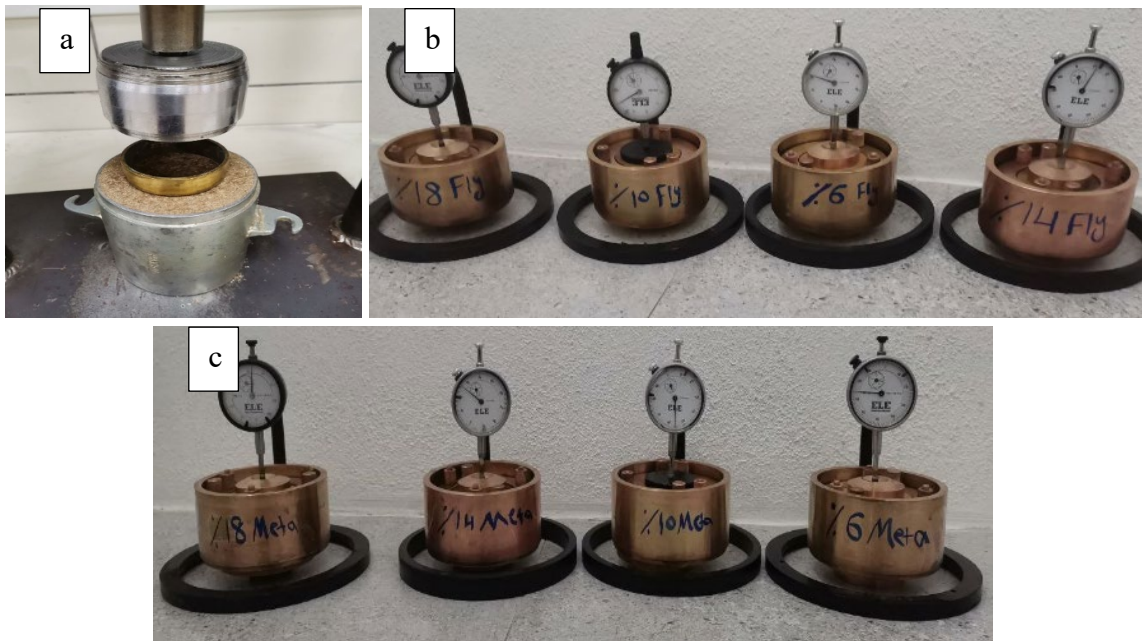
Figure 4: Swell-shrink potential of CH soil: a: pressing consolidation ring through compacted soil in compaction mold, b: samples for 1-D swell-shrink cycles test of fly ash-geopolymer-treated CH soil, and c: samples for 1-D swell-shrink cycles test of metakaolin-geopolymer-treated CH soil.
