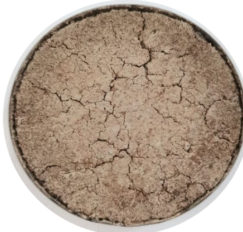
Figure 12b: 6% FA-geopolymer after 6 swell-shrink cycles.
