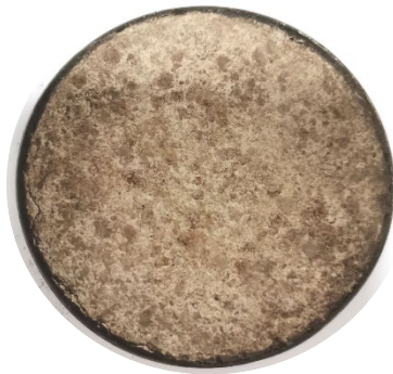
Figure 12d: 18% FA-geopolymer after 6 swell-shrink cycles.
