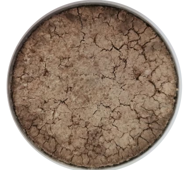
Figure 12c: 6% MK-geopolymer after 6 swell-shrink cycles.
