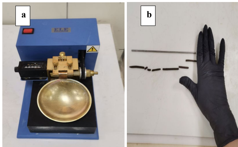
Figure 3: Atterberg limit tests, a: Liquid limit device; b: Plastic limit evaluation.
