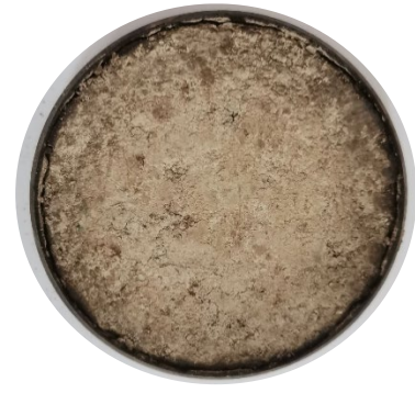
Figure 12e: 18% MK-geopolymer after 6 swell-shrink cycles.
