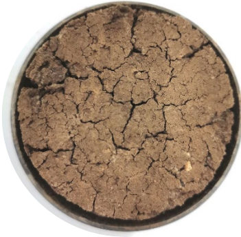
Figure 12a: CH soil after 6 swell-shrink cycles.
